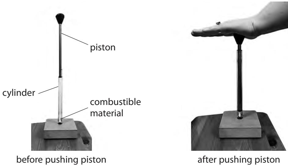
A small piece of combustible material is placed at the bottom of the cylinder.
